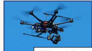
NASA Langley's Ultraviolet Corona Detection System
